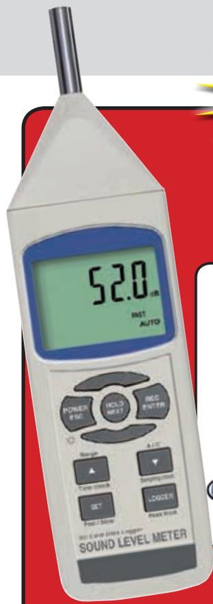
**DIGITAL SOUND LEVEL METER SD Card real time data logger**
